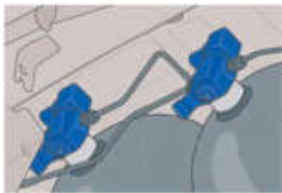
Electromagnetic shut-off valves on the gas tanks
